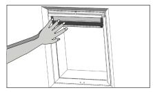
Hold the cassette in place until screws have been secured.
