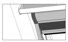
The siderail should be positioned underneath the front edge of the cassette.
