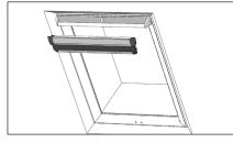
Position the cassette at top of the window frame and press firmly.
