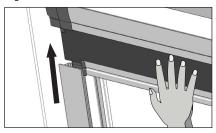
Slide fabric into the front channel of the siderail. Push siderail upwards.
