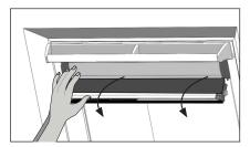
Flip handle and hold fabric flush with window.
