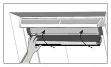
Pull handle away from the window and fold upwards against the front of the cassette.
