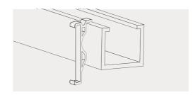
Open the gate of the box brackets and slide the headrail into position then snap the brackets closed.
