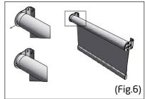
Then making sure the locating lugs on the end of the spring side is in the lowest position, place the blind into the spring end bracket. (Fig.5) Release the pin (do not pull all the way out) from the front side of the spring. Your blind has been pre-tensioned and is now ready to operate and will stop at the desired top position. (Fig.6)
