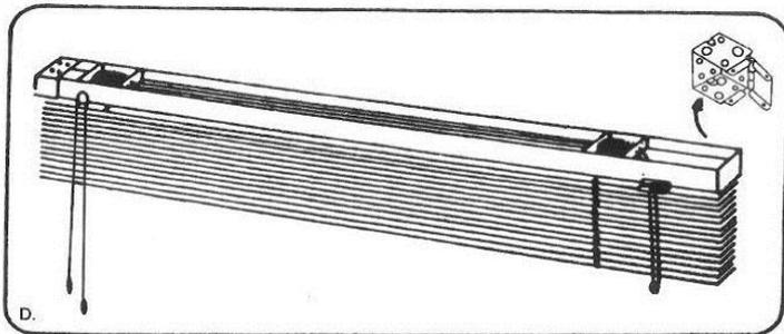
Correctly installed at 1.5m (60") from the floor, this supplied non-integral Child Safety Device is screw fixed & stores excess cord out of a child's reach.
