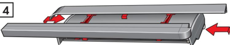
**English:** Remove end covers from both sides (**1**). Place adapter on axle and turn into position (**2**). Fix adapter with screw supplied (**3**). Refit end covers (**4**).
