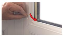
10. Push cord knot into hole, push fixing grommet into hole, aligning groove to cord.
