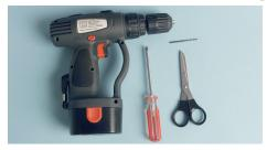
Fitting tools required include star point magnetic screwdriver (TP486), scissors and Ø2.5mm drill bit. (for TF see step b1 overleaf).
