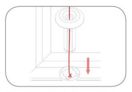
**6.** Insert the knot(s) on the loose cord into the pilot hole on the bottom bead followed by the bead grommet.
