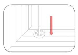
7. To secure the bead grommet ensure the cords are exiting the bead grommet towards you. Push the grommet until it is located fully. The cords should now be secured into the bead.
