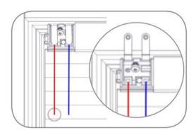
**8.** To tension blind, firmly hold the dangling cord from the headrail endcap and then open the gate. Repeat on the other side.
