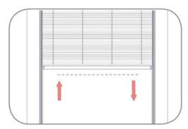
**10.** Test the tension by raising the blind, ensure it stays fully raised when released. Repeat the previous 2 steps if required. Ensure bottom bar is straight by adjusting it from side to side.
