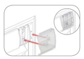
**12.** Attach endcap cover by aligning the clip on the side with the clip on the endcap. Push the endcap in fully until a click is heard.
