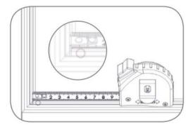
**3.** Mark 6mm from the bottom corner of the frame. Repeat this on the other side.
