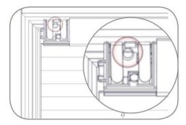
1. Place your blind against the frame of your door or window ensuring the back of the blind is parallel to the glass and the endcap sits comfortably on the bead. Place a small mark where the centre hole of the endcap is. Repeat this for both headrail endcaps.
