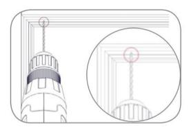
**2.** Using your mark as a guide. Drill into the bead at 45°. Repeat this process on the other side. (2.5mm drill bit).
