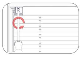
**5.** Line the blind up with the pilot holes in the top bead. Using the screws provided, screw the blind to the bead of the window/door.
