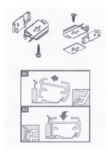
2b. Install head rails with sliding tensioners in a similar manner to the head rail as shown in point 2a, but you will need to fit with a minimum of one packing shim behind each bracket to allow for the sliding tensioners.
