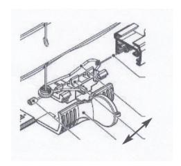
4. The operating cords are also tied off to a sliding tensioner and can be adjusted in the same way, to create the optimum tension to hold the blind in place without being too much to make it stiff to operate.
