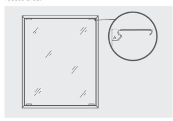
Complete this for the top and the bottom of the blind. The installation brackets (top and face fix) are positioned evenly along the width of the blind. Hold each bracket into place and mark the hole positions. Please ensure fixings are suitable for the wall/surface to which you are mounting the brackets.
