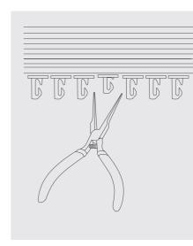
the headrail have been pushed in, if they have, using a pair of pliers, gently pull the pegs back out.
