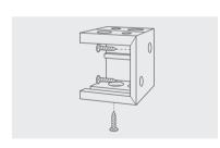
Open the gate of the box brackets and slide the headrail into position then snap the brackets closed.
