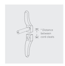
Mark the hole positions and drill as required.
